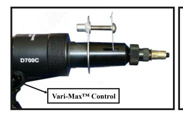
The **D-700-VM Vari-Max<sup>TM</sup>** feature enables the user to set a pull force when upsetting a blind rivet nutor insert to help insure a proper installation without damaging the threads of the blind nut insert or the threads on the pull-up stud. The normal operating range for the D-700-VM is 1000 to 5,000 lbs. The Vari-Max<sup>TM</sup> is located on the tool on the side opposite the release button (right side of the tool facing forward).
